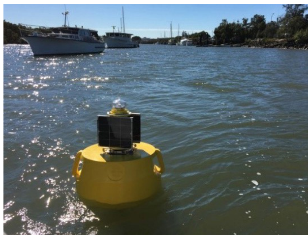
Real-time water quality monitoring buoy (YSI DB-600)
